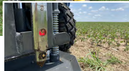
No ground engaging components, except at probe locations, creates a wide mapping window for the Veris’ CoreScan. Photo: Veris Technologies
